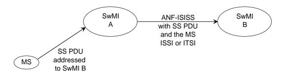
Figure 1: SS PDU addressed by a MS to a distant SwMI
