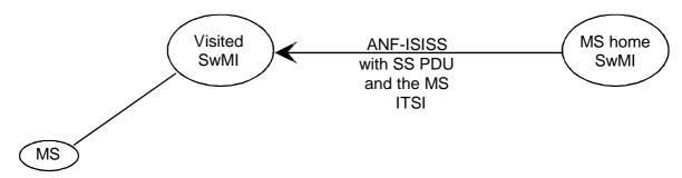
Figure 2: SS PDU addressed individually by a home SwMI to a MS having migrated
