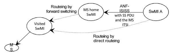
Figure 3: SS PDU addressed individually by an SwMI to an MS
